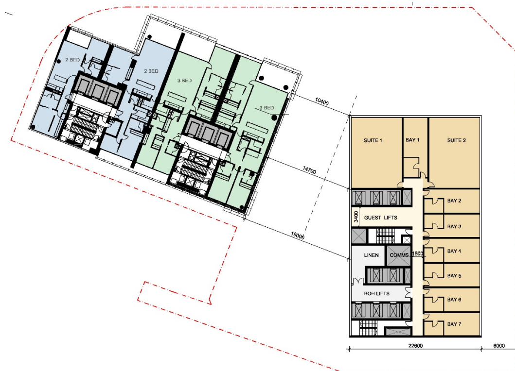
Figure 25: Building separation between amended proposal (left) and Stage 1 DA indicative plan for Building B
